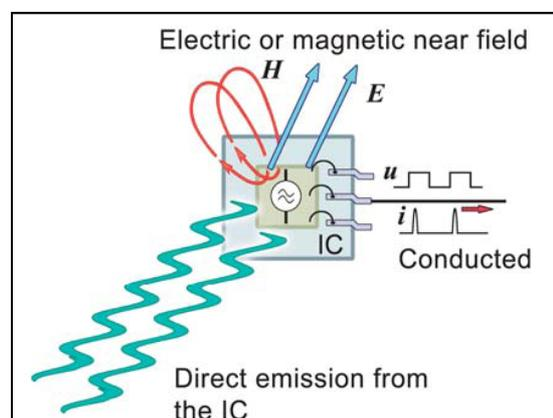
Fig. 1. Ways how an IC generates disturbances
