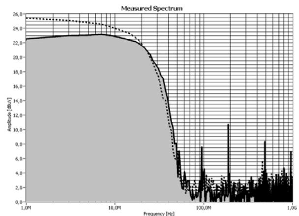
Fig. 10. Loop measurement with the RFB 0,3-3 magnetic field probe vs. reference
