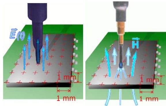
Fig. 6. Near electric and magnetic field probes for the characterization of the electromagnetic emission of integrated circuits.
