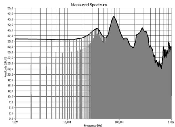
Fig. 13. Measurement result of an IC – TEM cell method (reference)
